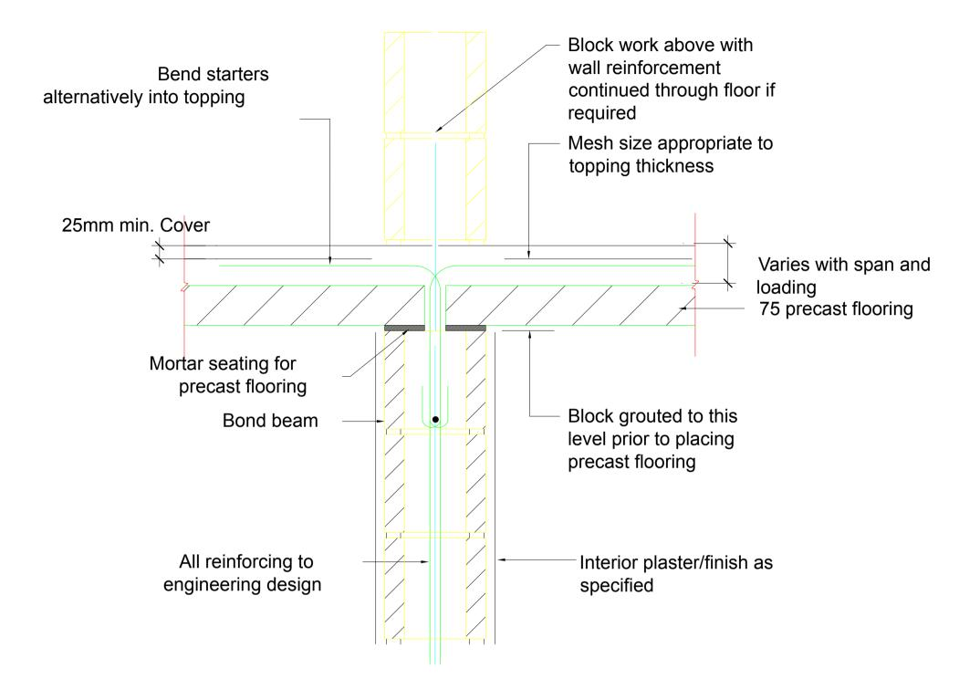
Unispan Intermediate Support Scale 1:10
